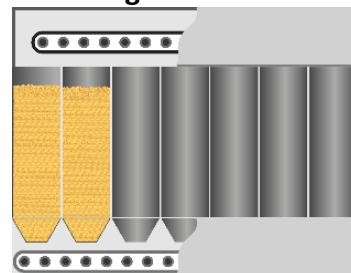
Vertical grain storage facilities (silos) are the most technologically advanced and offer the highest productivity. Vertical grain storage facilities (silos) are the most common worldwide. Grain storage heights typically range from 6 to 30 meters.
